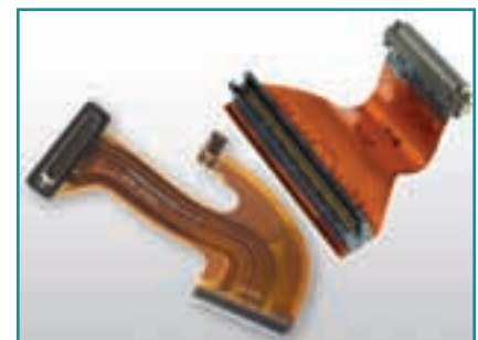
FLEX CIRCUITRY WITH RECTANGULAR CONNECTORS
