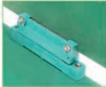
DB to MB Mating Boards at Right Angles
