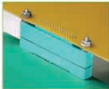
MB to I/O-P Mating Parallel Boards
