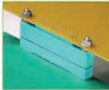
MB to I/O-P Mating Parallel Boards
