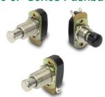
The 16-3P-Series pushbutton switches are single pole and AC rated up to 3 amps. These momentary action switches have a slow-make, slow-break contact mechanism and require only light actuation force (4 oz. - 1 lb.). These switches are typically used in general purpose applications requiring finger actuation.
