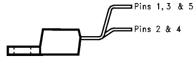
Side View LM2575T-XX Flow LB03 or LM2575HVT-XX Flow LB03 See NS Package Number T05D
