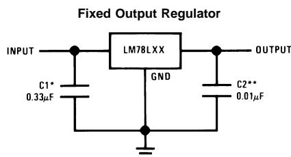
\*Required if the regulator is located more than 3" from the power supply filter.
