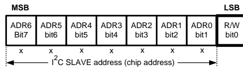
Figure 16. I 2 C Chip Address (0x2C)
